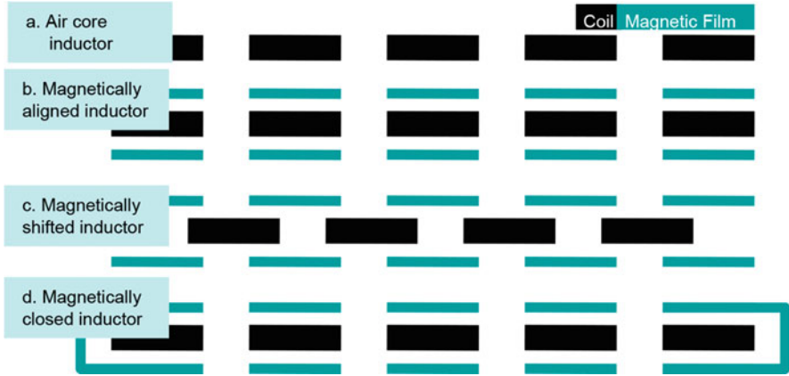
Fig. 10.9 Cross-sectional view of relative position of magnetic film with respect to the spiral leg [5]
