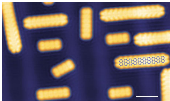
Fig. 23.13 STM image of graphene nanoribbons of different lengths obtained with a fabrication technique based on-surface polymerization. (Reproduced from Kimouche et al. [96])
