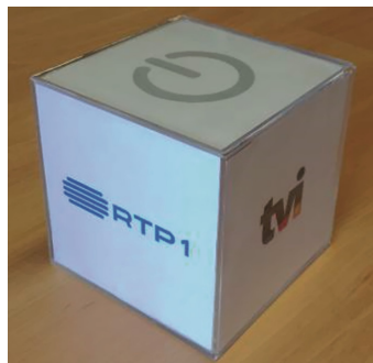
Fig. 1. The SIX with personalized paper labels (standby symbol and channels logos)
