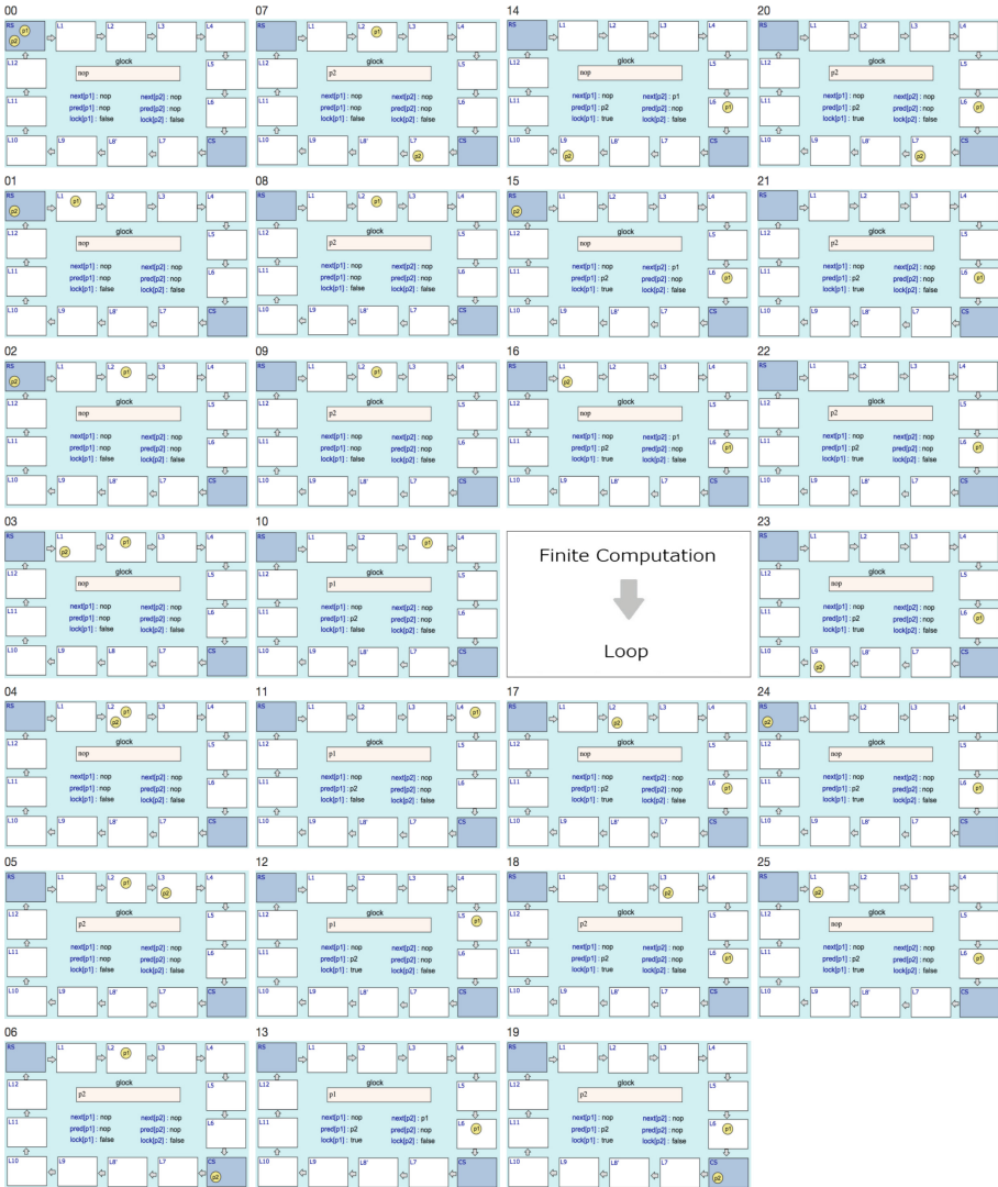
Fig. 8. A counterexample for the lockout freedom property for MCS protocol in which comp&swap is not naively used.
