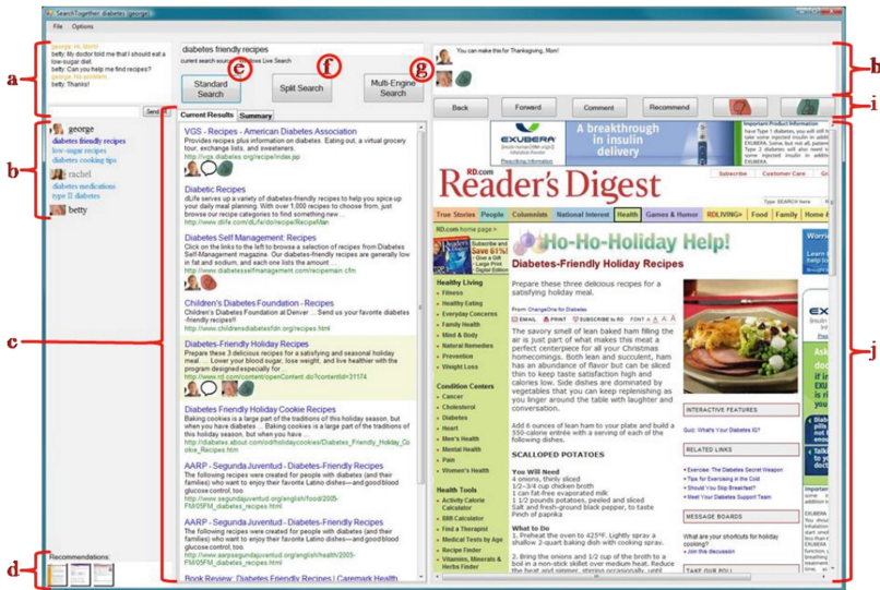
Fig. 5. The SearchTogether system: (a) integrating messaging, (b) query awareness, (c) current results, (d) recommendation queue, (e)–(g) search buttons, (h) page-specific metadata, (i) toolbar, (j) browser. (Adapted with permission from Morris and Horvitz [48].)
