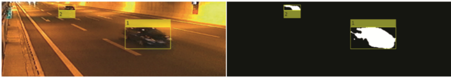
Fig. 8. Blob tracking based on foreground detection
