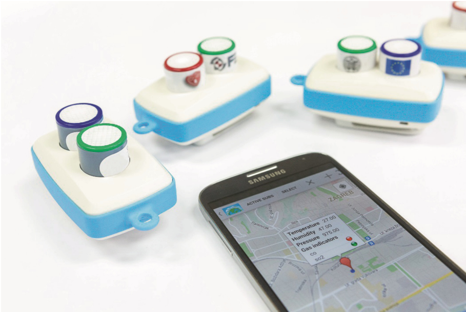
Fig. 3. Wearable sensors for air quality monitoring (Wearable sensors and smartphone application for air quality monitoring developed at University of Zagreb, Faculty of Electrical Engineering and Computing, Zagreb, Croatia.)
