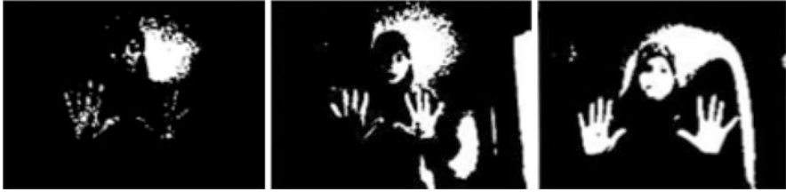
Fig. 3 Skin detection results based on HSV, YCbCr, and RGB color spaces, respectively
