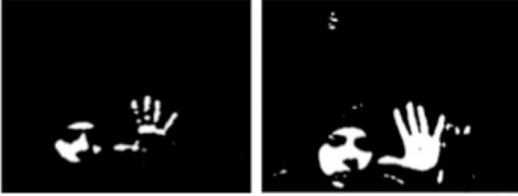
Fig. 4 RGB mask before and after the correction, under a brightness between 70 and 190
