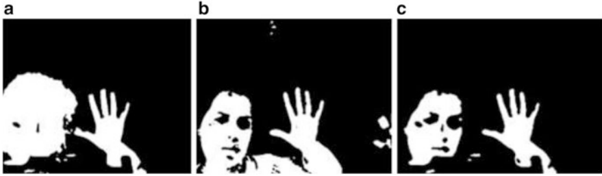
Fig. 2 (a) Foreground subtracted (b) RGB mask applied in the input image (c) AND operation
