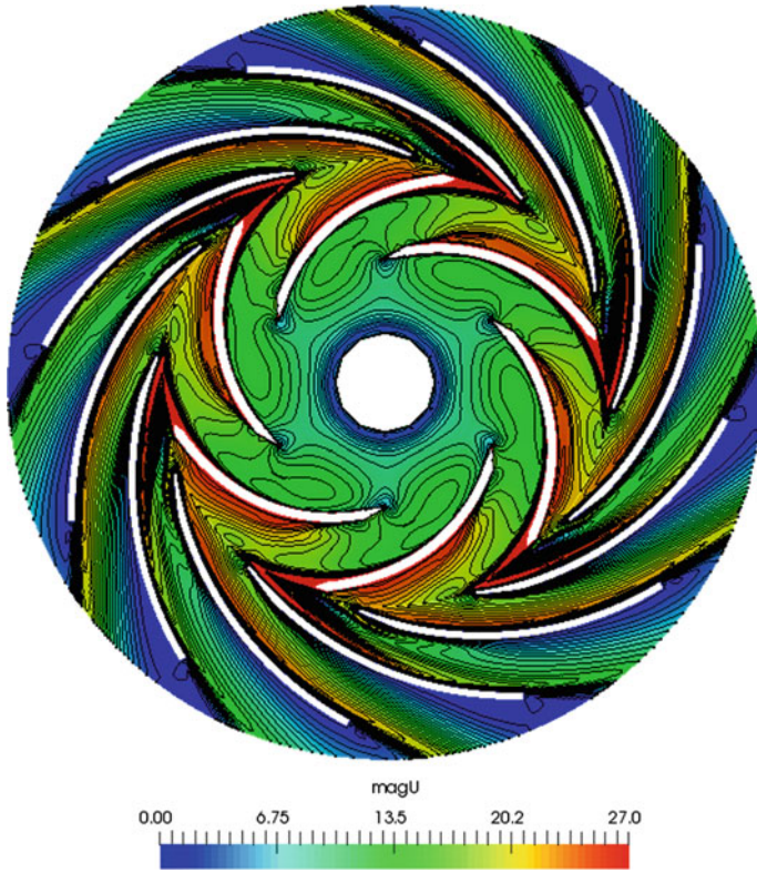
Fig. 19 Velocity magnitude contours of the optimal impeller at span 50%
