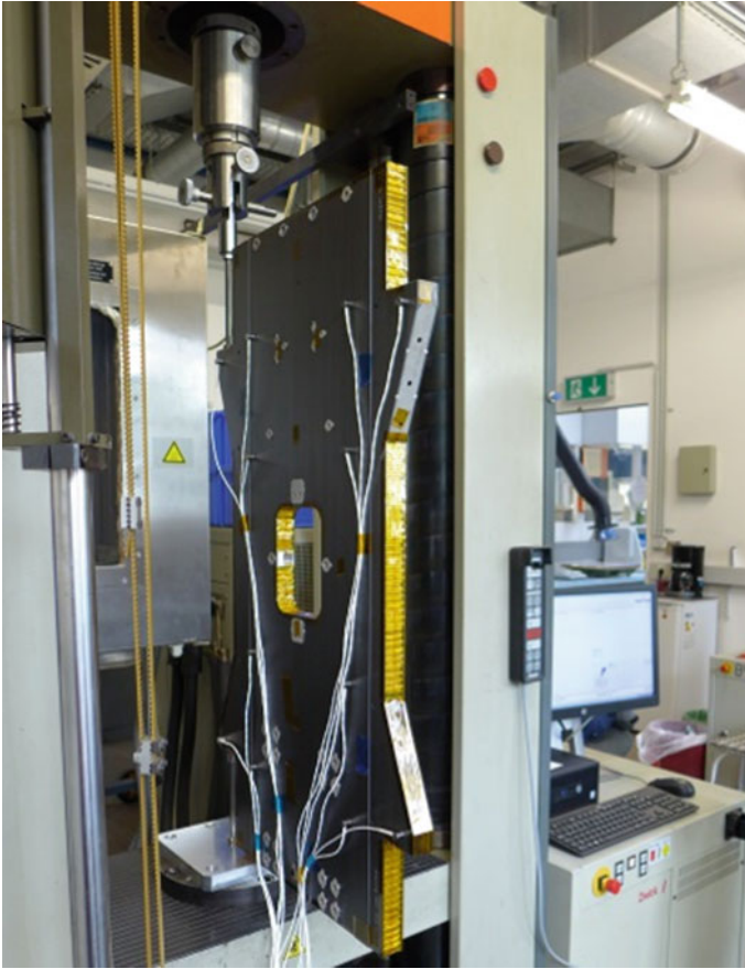
Fig. 13 Panel insert breadboard in tensile test machine
