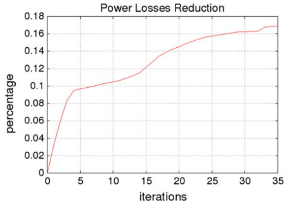
Fig. 8 Optimized sBend duct shape, achieving a 17.1% power losses reduction
