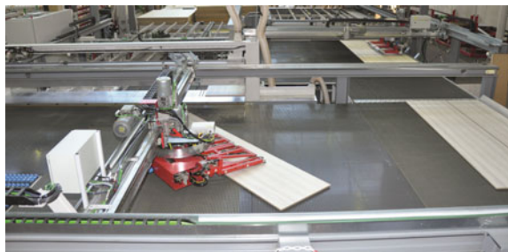
Fig. 1 Gantry robot transporting a panel outputted by a saw towards other panels on a feedback conveyor
