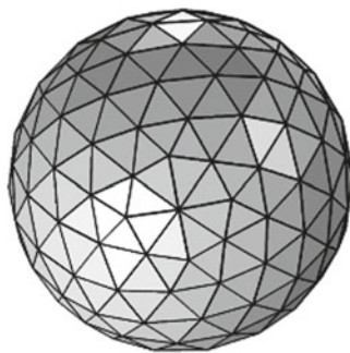
Fig. 3 Discretized sphere model for evaluation of discrete mean curvatures
