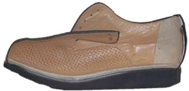
Fig. 27.4 Section of a shoe with “biomechanical properties”: the recessed heel allows a soft impact at heel strike; the point of rolling inserted immediately behind the metatarsal heads allows a smooth transition from midstance to propulsion; the presence of a wider angle between the sole and the ground at the most anterior part of the shoe further reduces the stress at the level of metatarsal heads during propulsion and toe-off
