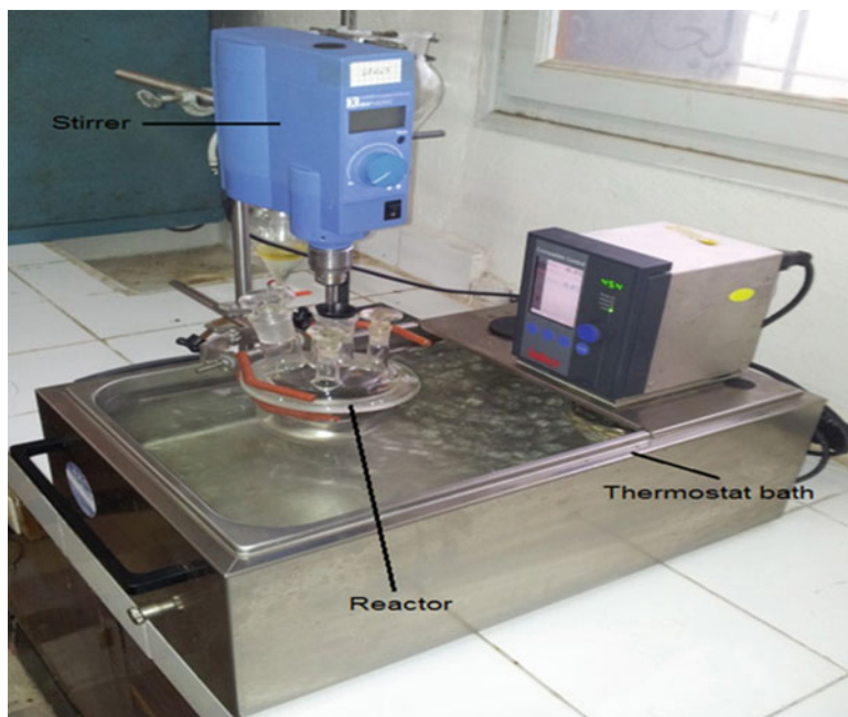
Fig. 32.1 Experimental setup for transesterification reaction
