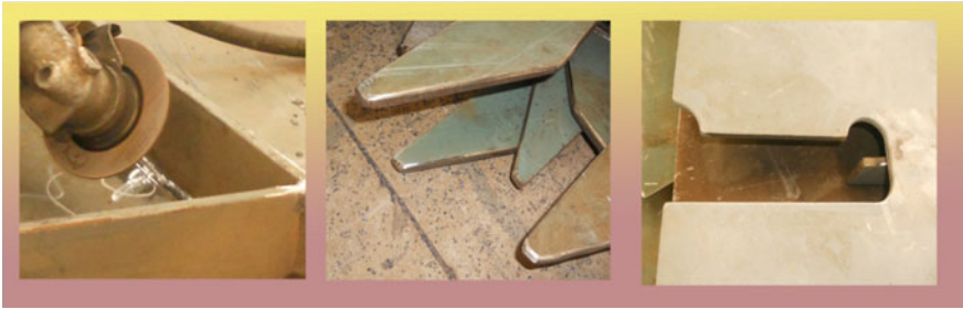
Fig. 3 Rounded edges (R-2 mm), according to the standard, before assembling the block sections
