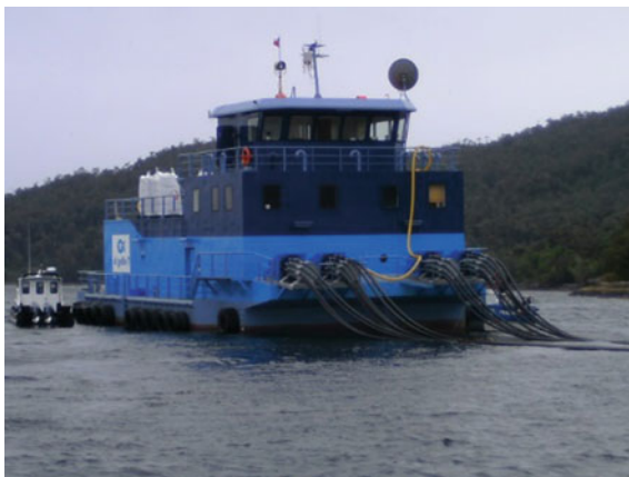
Fig. 10 Control and feeding pontoon
