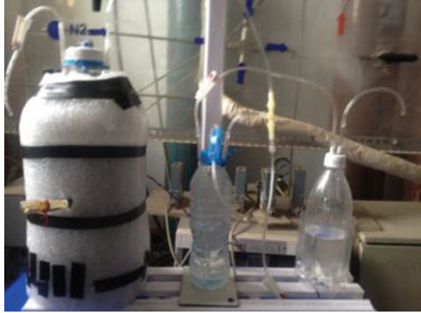
Fig. 4 A photo of the anaerobic digestion system used in this study
