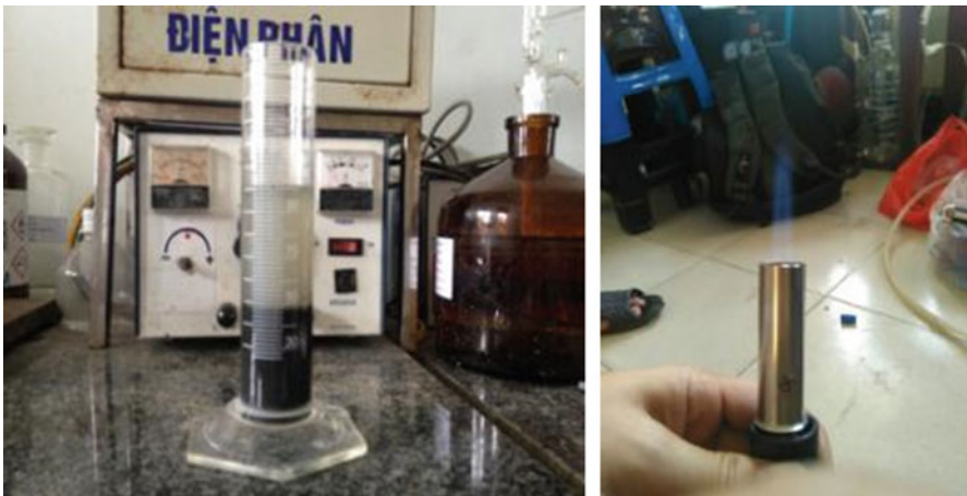
Fig. 14 A photo of sludge after anaerobic digestion (left) and biogas generation burned (right)
