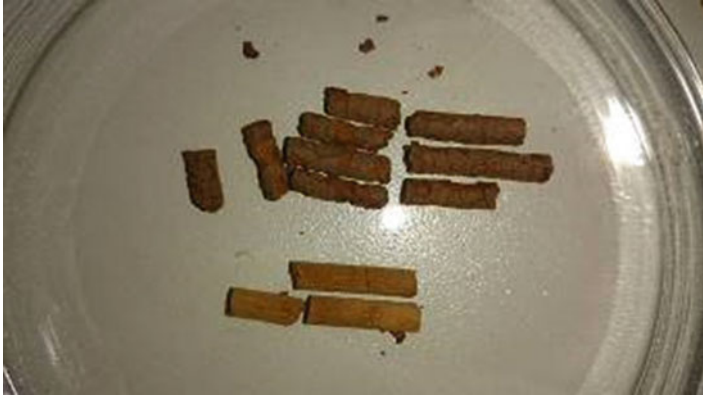
Fig. 11 Adsorbent after H 2 S purification and contact with air for about 1 h
