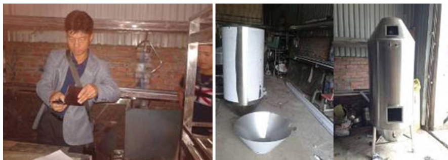
Picture 6 Adsorbent tower was designed and manufactured
