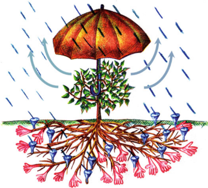
Fig. 1 Soil stabilising functions of plants, e.g. interception, evapo-transpiration, and root reinforcement
