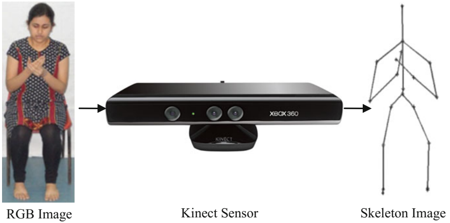
Fig. 2 RGB image with its corresponding body joints as recognized using Kinect sensor
