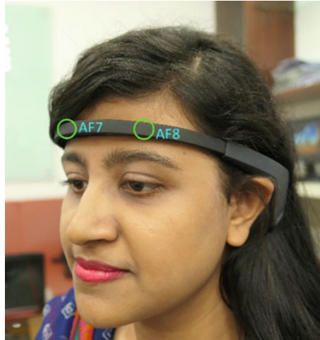
Fig. 4 AF7 and AF8 channel locations of the Muse headband
