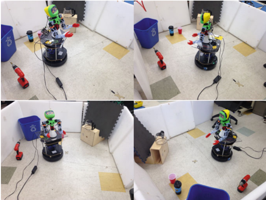
Fig. 9 Redesigned prototype of the system with the mobile platform and the torso robot is installed performing object identification and navigation tasks
