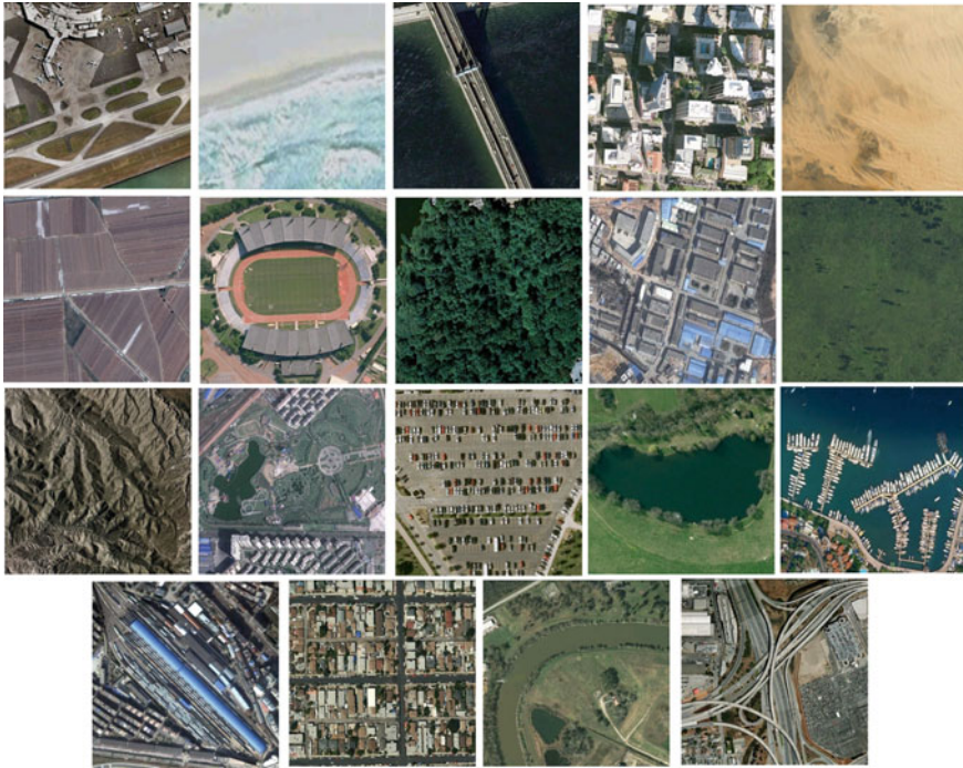
Fig. 9 Sample image chips from the 19 class RSD benchmark dataset, each 600 \times 600 pixels of various spatial resolution. Classes in left-to-right, top-down order: 1 airport , 2 beach , 3 bridge , 4 commercial area , 5 desert , 6 farmland , 7 football field , 8 forest , 9 industrial area , 10 meadow , 11 mountain , 12 parking lot , 14 pond , 15 port , 16 railway station , 17 residential area , 18 river , and 19 viaduct . In Sect. 5.2, neuron indices are used instead of text descriptions for sake of compactness
