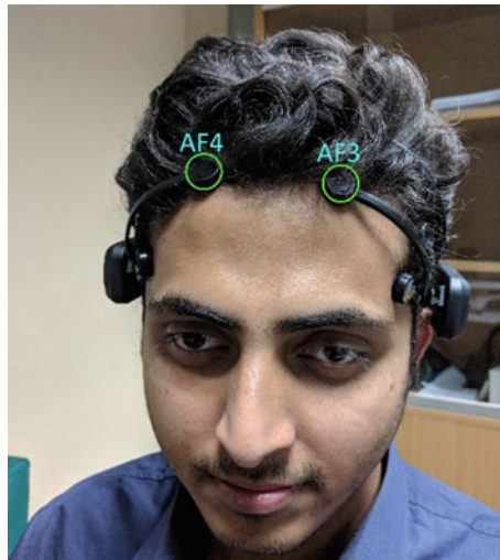
Fig. 5 AF3 and AF4 channel locations of Emotiv EPOC
