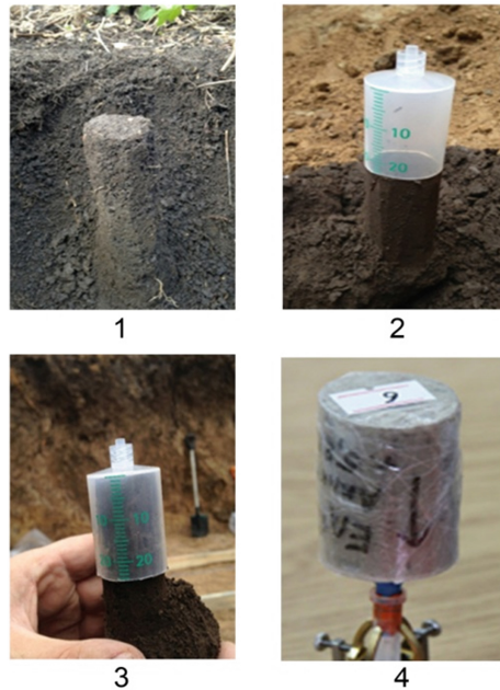
Fig. 1. Soil sampling for tomographic study.
