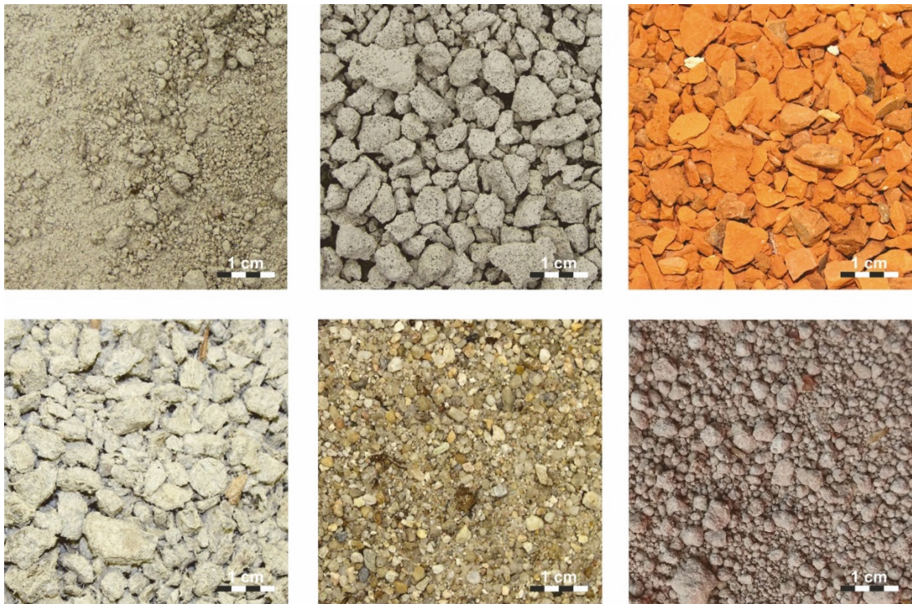
Fig. 1. Selected technogenic materials analysed in the paper: neat plaster, aerated concrete, bricks, asbestos-cement roof plank, building sand and municipal sewage sludge
