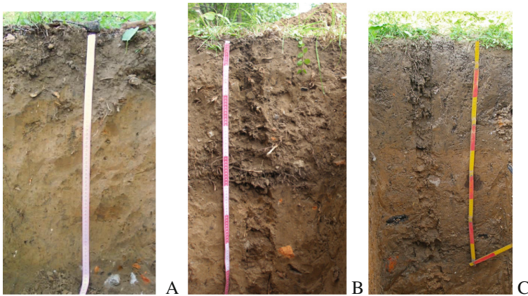
Fig. 2. Urbic Technosols: A. - postlithogenic; B. and C. - sinlithogenic on the Lomonosov Moscow State University campus.
