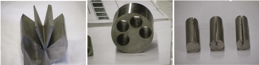
Fig. 4. Cutting results and surface quality for abrasive waterjet cutting
