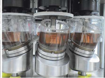
MTS 8-station hip simulator (Eden Prairie, MN, USA)
