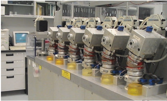
AMTI 12-station hip simulator (Water Town, MA, USA)
