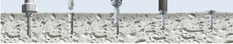
Fig. 12 Pre-drilling, insertion, fusion, and the resultant fixture when the SonicWeld Rx ® is used. Image courtesy of KLS Martin
