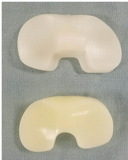
Fig. 2 The differences in a standard highly cross-linked polyethylene (top) and a Vitamin E infused highly cross-linked polyethylene (bottom) total knee inserts, showing the yellow coloration caused by the Vitamin E infusion. The goal of vitamin E is to stabilize the material to prevent oxidative degradation of the polyethylene. This also provides increased strength as additional steps of remelting are not required thereby reducing crystallinity
