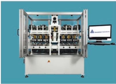
PROSIM 6-station hip simulator (Simulation Solutions, Stock Port, UK)
