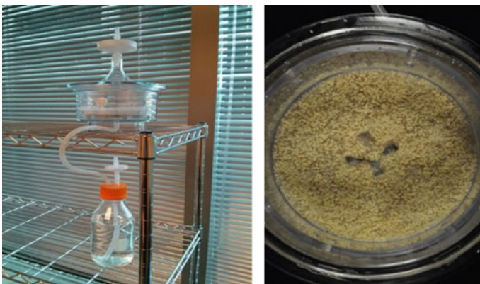
Fig. 1 The new temporary immersion bioreactor-model developed primarily for conifer SE. Mature somatic embryos of Norway spruce in bioreactor (top view)
