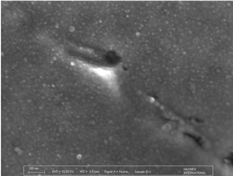
Fig. 3 Very high magnification SEM in-lens photomicrograph of the 282 alloy sheet samples in the initial, mill-annealed condition indicating the presence of very fine cooling \gamma'
