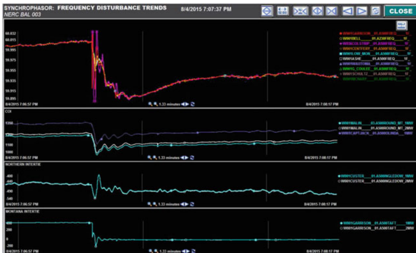
Frequency disturbance trend display provides a synchronized view of the system frequency and active power flows on BPA-operated interties during a frequency deviation event
