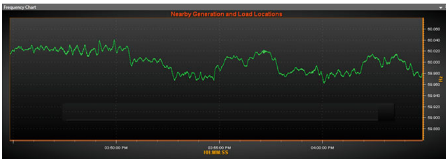
Fig. 7.3 No oscillations in March after controller replacement
