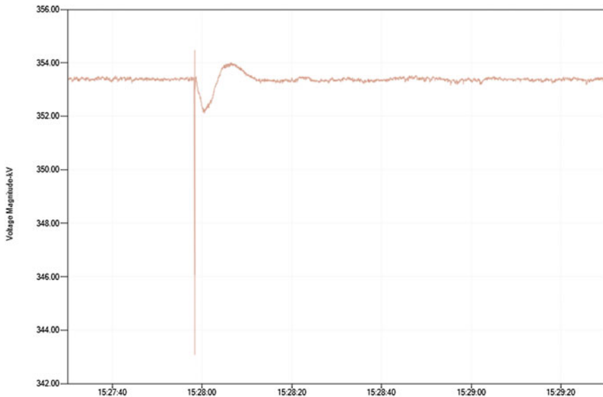
Fig. 15.2 PMU with largest voltage drop due to fault
