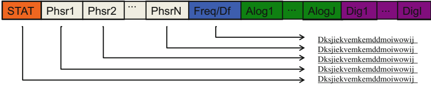
Fig. 2.5 Data is sent as a string of values and has to be parsed using a matching guide
