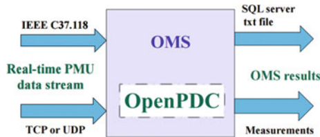
Fig. 9.10 Block diagram of WSU OMS tool
