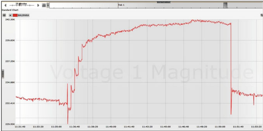
Fig. 17.23 Positive sequence voltage magnitude (first instance)
