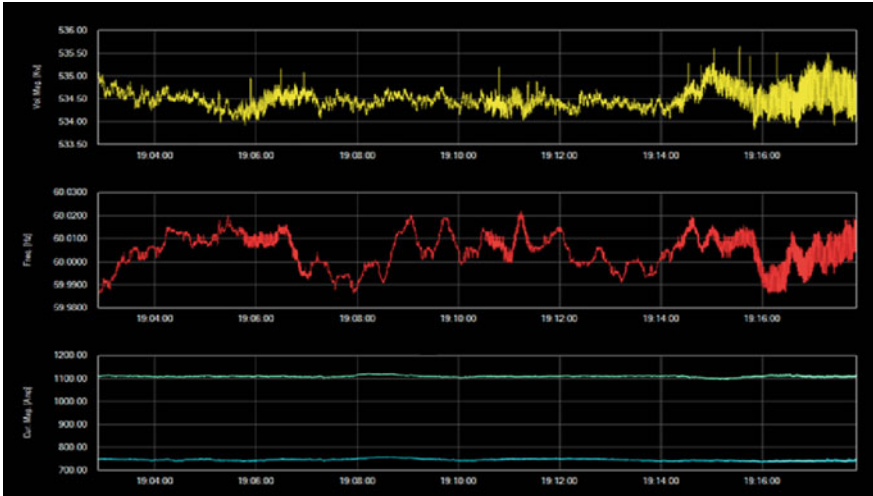
Fig. 11.5 High-frequency solar plant-based local oscillation event
