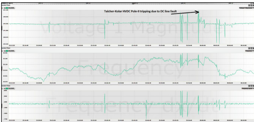
Fig. 17.33 PMU voltage plot indicating transients due to DC line faults
