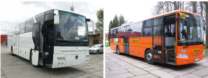
Fig. 3 Folding door (circular sliding movement) outside the bus
