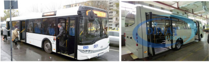
(a) Fully folding doors inside the bus (b) Partially folding doors inside the bus
