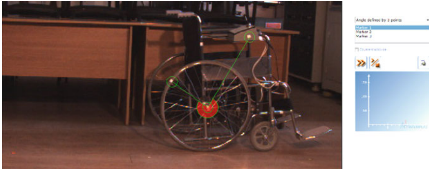
Fig. 12 Wheelchair marker tracking for computation of angular velocity of the wheels
