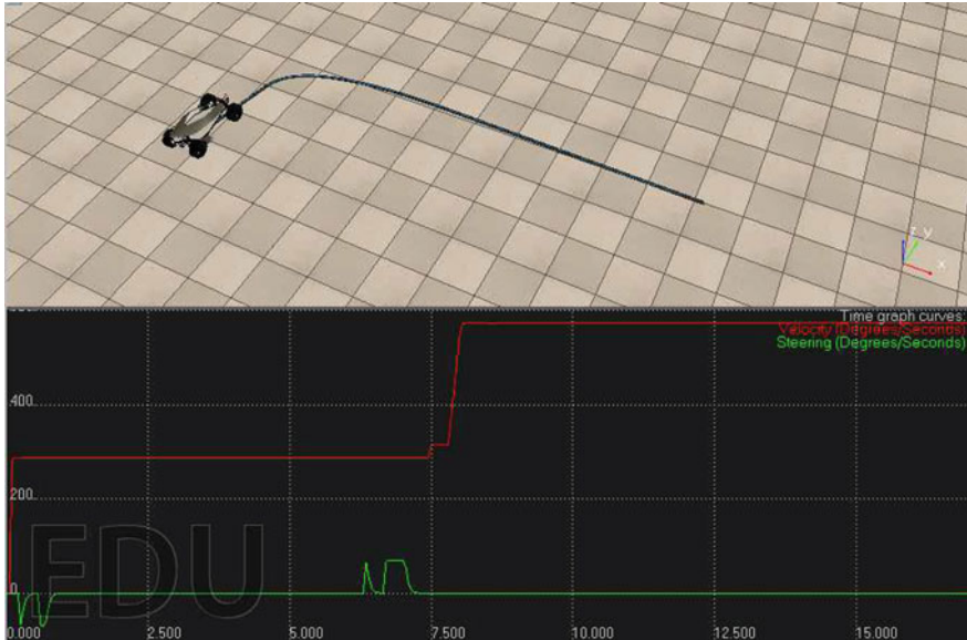
Fig. 4 Velocity variation analysis when the vehicle accelerates while steering in a industrial narrow environment
