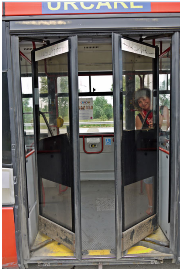
Fig. 5 a Fully folding doors inside the bus. b Partially folding doors inside the bus
