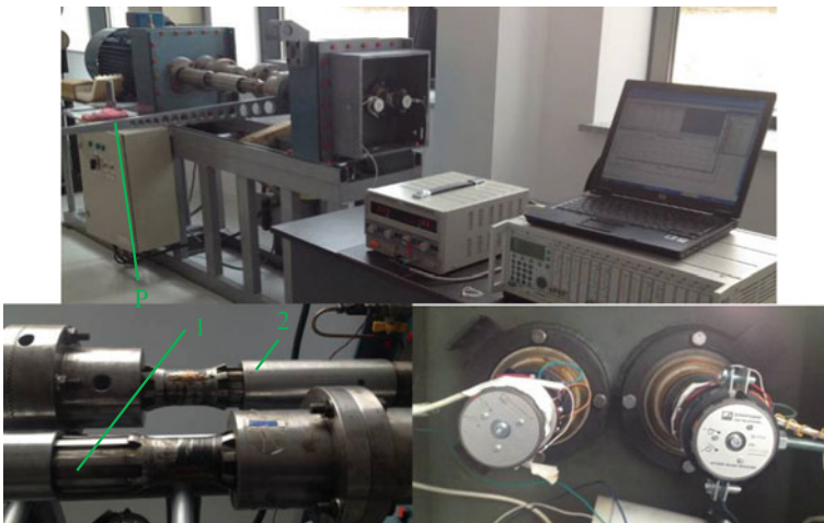
Fig. 3 Experimental model of the spur gears efficiency test bench
