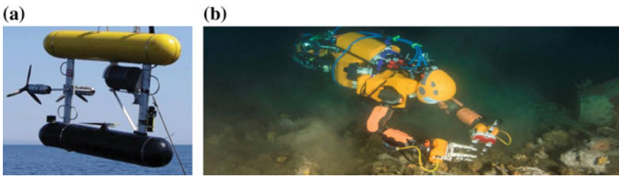
Fig. 3 Robots for undersea exploration: a SeaBED AUV, [8]; b Ocean One, [12]
