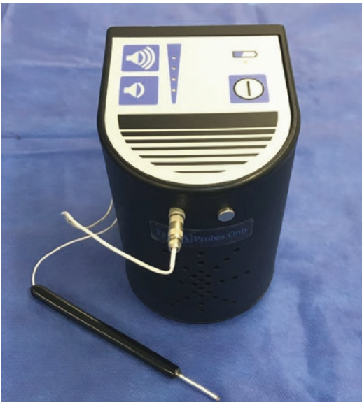
Fig. 35.2 9.3 Mhz VTI surgical Doppler (Vascular Technology Int., USA) and a disposable probe flow detector
