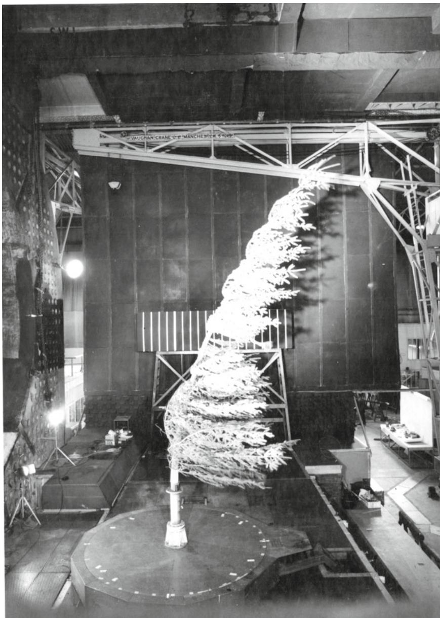
Fig. 4 Reconfiguration of the crown of a Sitka spruce tree in the Royal Aircraft Establishment wind tunnel at a constant wind speed of 24.9 m/s. Photograph from Graham Mayhead © Crown Copyright Forestry Commission. Used with permission. For details of tests see Mayhead (1973)
