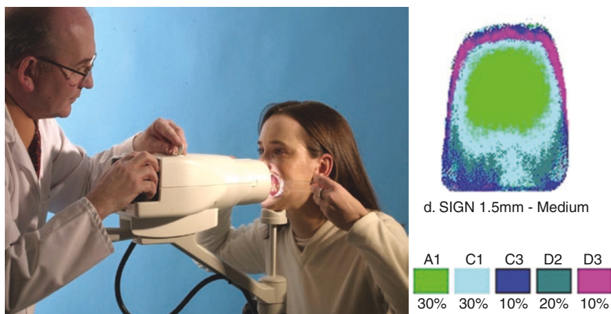
Fig. 17.6 The Ikam™ (Metalor Technologies SA), a pioneering digital camera-based system for shade analysis. The screen image (right) gives a two-dimensional representation of the selected ceramic shades
