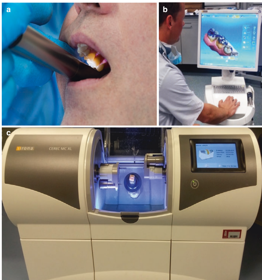
Fig. 14.1 (a) Data acquisition via digital scanning to record an optical impression followed by information transfer; (b) data processing to design a virtual form of the restoration/coping using computer software; (c) manufacturing —a machine receives the processed data and manufactures the restoration/coping. This Cerec™ machine can mill blocks of alloy, ceramic or composite. Its size is mid-range suitable for laboratories. There are smaller machines for chairside use and much larger ones weighing several tonnes for milling centres (Courtesy of Andrew Keeling)
