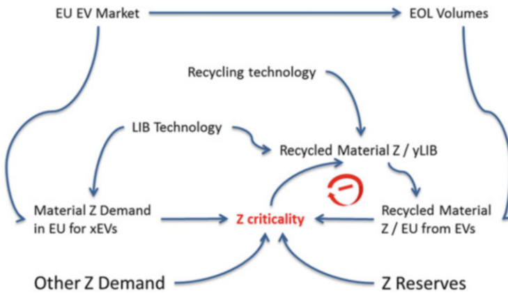
Fig. 5 Simplified SD diagram regarding the dynamic of minerals consumption for LIBs in Europe
