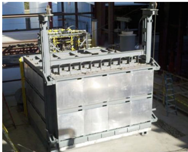
Fig. 2 A forge furnace developed by our industrial partner
