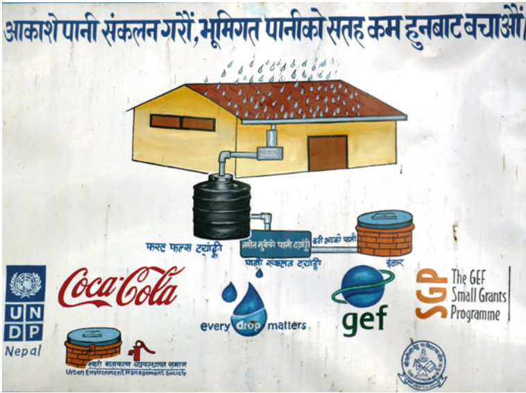
Fig. 4.10 Rainwater harvesting to individual well (Source Author)
