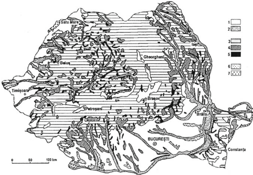
Fig. 5.5 General map of soil erosion in Romania. Erosion-free lands : 1 without flood risk; 2 flood and alluvial risk; areas affected by water erosion : 3 low erosion but accelerated erosion risk, 4 moderate strong erosion with accelerated erosion risk, 5 very strong, excessive erosion; terrains affected by wind erosion : 6 moderately strong erosion at risk with accelerated erosion; 7 very strong, excessive erosion. (Florea et al. 1999 with modifications)
