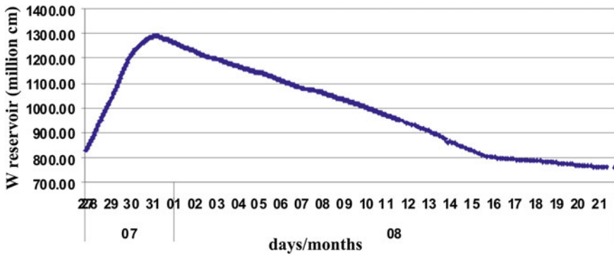
Fig. 6.9 Evolution of water volume within the Stanca–Costesti Hydro-Energetical Junction during the backwater in the summer of the year 2008. Source Author
