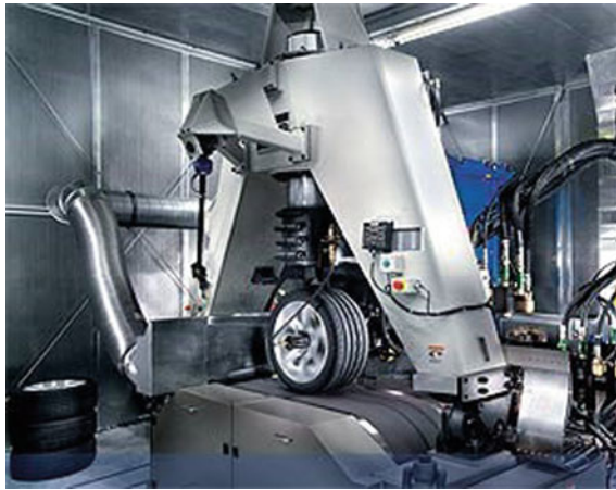
Fig. 6 IABG Flat-Trac tire force and moment testing machine
