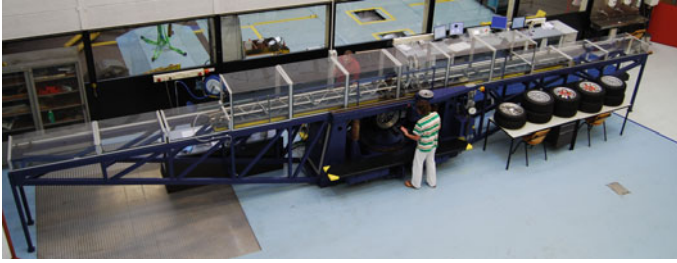
Fig. 34 TU/e flat plank tire tester
