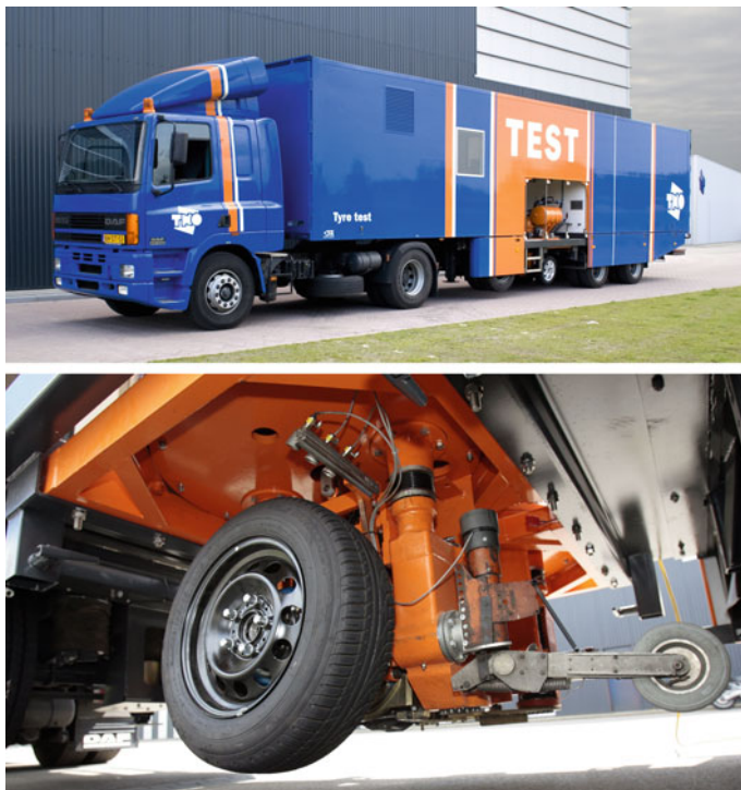
Fig. 7 TASS tire test trailer
