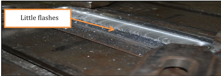
Fig. 5 Surface appearance of friction stir processed surface at 400 rpm and 100% SiC
