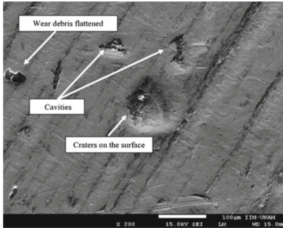
Fig. 15 Wear mechanisms (trailing edge) with scale of 100 micrometers and show craters and cavities
