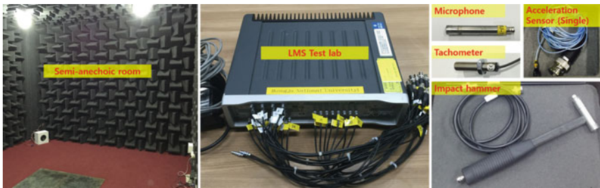
Fig. 2 Test room, measurement/analysis system and sensors
