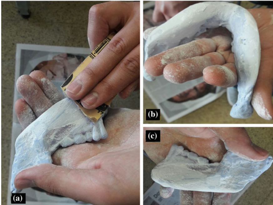
Fig. 6 Reduction of the body's surface and the mandibular branches using sandpaper, grain 80, a upper view of the lower jaw's left, lateral body, b smoothing of the inner body's surface and the mandible's base, removal of the anatomically deformed areas which altered the natural mandible's geometry, c lateral view of the mandible's body after 5 min of smoothing
