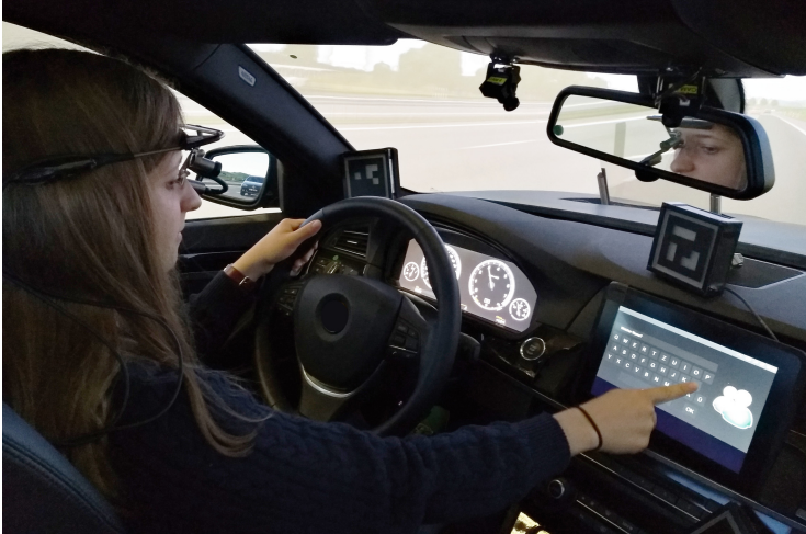
Fig. 3. The cockpit in the experimental setup. The experimental tasks were displayed on the central display and participants decided whether to use touch or speech for interaction. Glance behavior was recorded using a head-mounted eye tracker.
