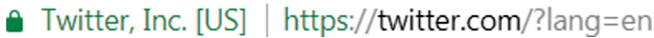
Fig. 2. EV in Chrome: green padlock, company name, country of origin, and “https,” (Color figure online)
