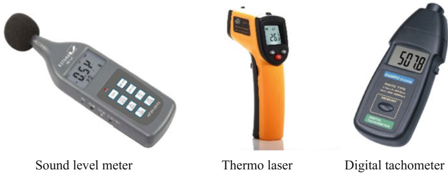
Fig. 50.2 Tools used to measure squeal noise, rpm, and temperature
