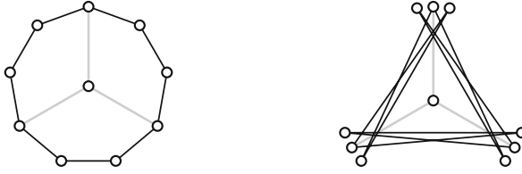
Fig. 2. Left: The graph H(k) . Each circle represents k independent vertices, each black line segment represents a bundle of k^2 edges, each gray line segment represents k edges. Right: A non-convex drawing of H(k) .
