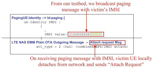
Fig. 10. The network and UE logs show that the paging message with victim’s IMSI can detach the victim device from the network
