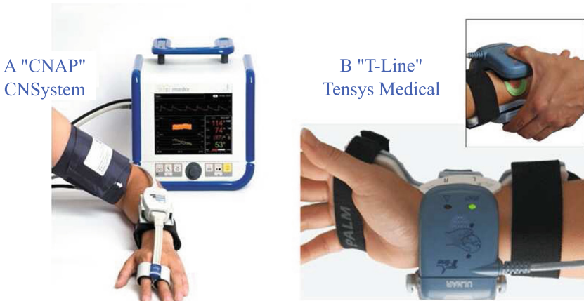
Fig. 1. Modern approaches to continuous ABP monitoring. (A) CNSystem TM CNAP device, employing the Penaz’s volume clamp method, (B) T-Line device from Tensys Medical TM based on arterial tonometry method
