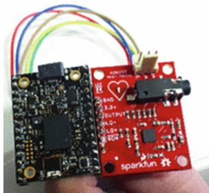
Fig. 6. Microelectronic for testing the prototype. Left a TinyTILE and right an ECG-board from Sparkfun.
