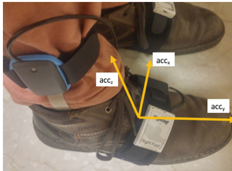
Fig. 1. Instrumented shoe setup with axes orientation
