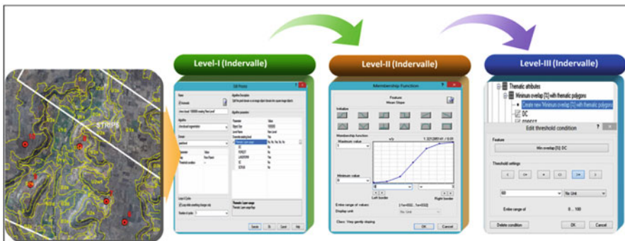
Fig. 9.3 Hierarchical object-based segmentation algorithm process for generating LEU maps
