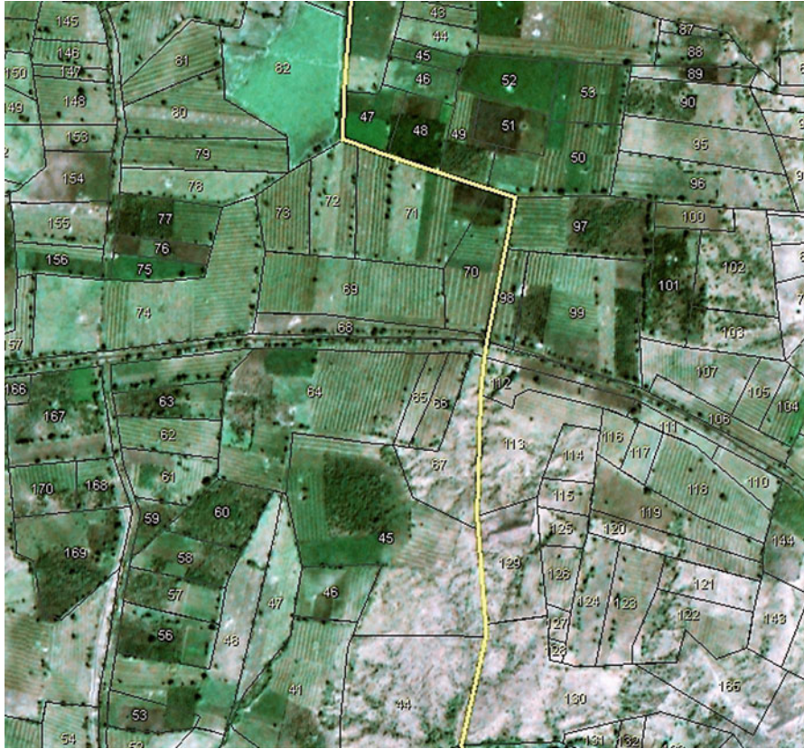
Fig. 29.1 Georeferenced village cadastral map of part of Chandur Bazar Taluk, Amravati District, Maharashtra, overlaid on the natural color composite high-resolution satellite merged product of Cartosat-1 (PAN) and Resourcesat-1 LISS-IV (multispectral). The yellow line is the boundary between Masod & Tonglapur villages, and the grey lines are the parcel boundaries with the parcel numbers
