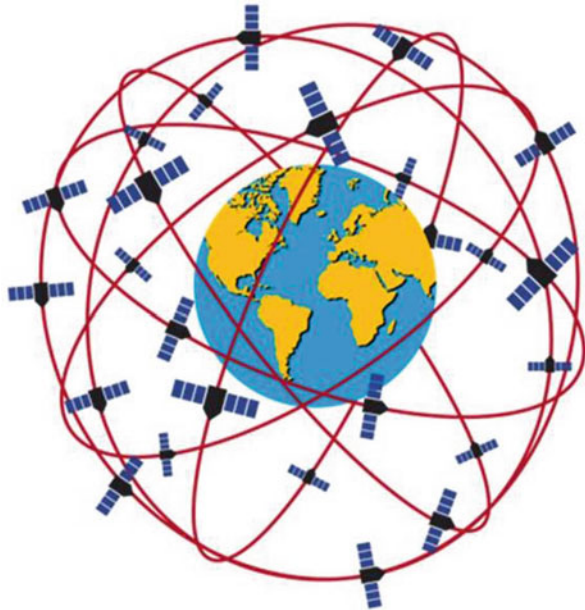
Fig. 4.1 Constellation of GPS satellites
