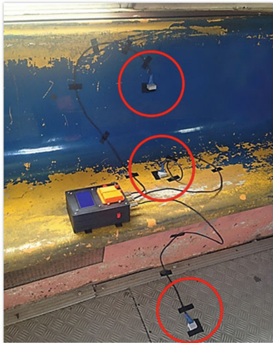
Fig. 3 Arrangement of the monitoring device in the train bench
