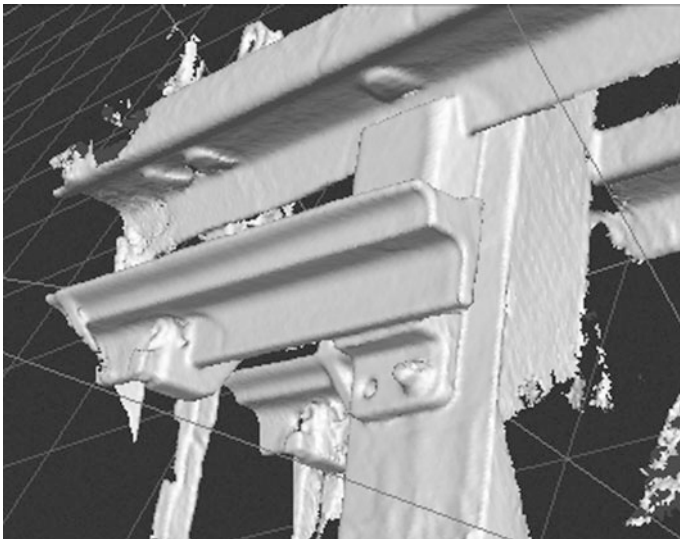
Fig. 6 3D model of intact UIC60 turnout blade in 300 radius scanned by Kinect device
