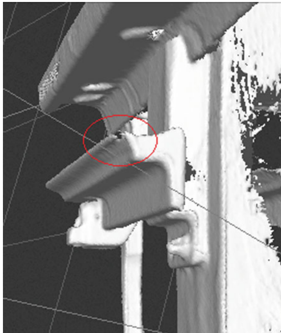
Fig. 7 Damaged UIC60 turnout blade in radius 300 while scanning by Kinect device
