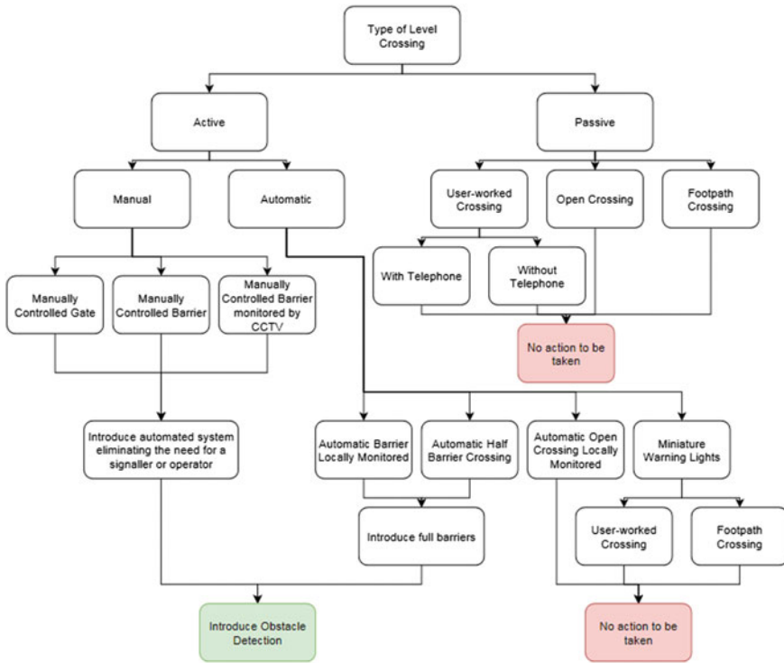
Fig. 18 A flow chart to show a generic outline of what should happen at each current type of level crossing
