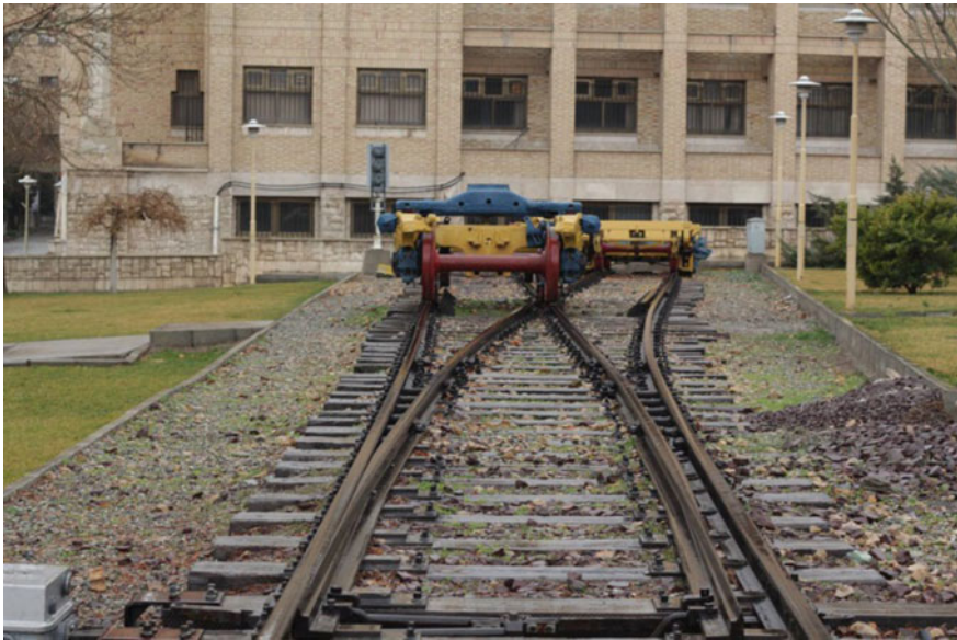
Fig. 2 Turnout of IUST used in experimental model
