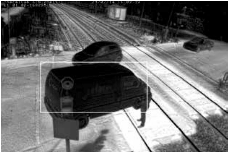
Fig. 12 An image captured by thermal imaging which shows a clear contrast between pedestrians and vehicles with the background (FLIR 2016)
