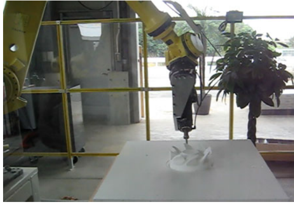
Fig. 2 Machining robot based on FANUC R2000iC
