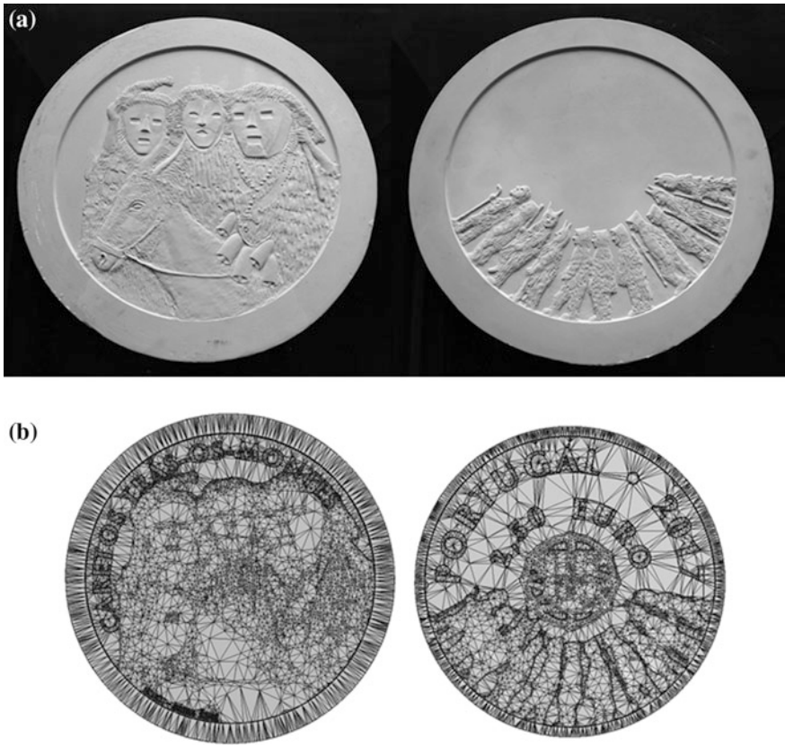
Fig. 2 Discretization of the die surfaces. a Original clay models supplied by the sculptor (scale 7:1) and b discretization of the die surfaces by means of spatial triangular elements after scanning and scaling down the clay models to the actual coin size
