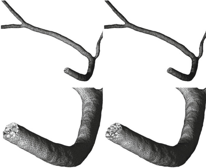
Fig. 1 The coarse (63k, left) and fine (120k, right) grids in the right coronary artery. The bottom figures zoom a part of the domain
