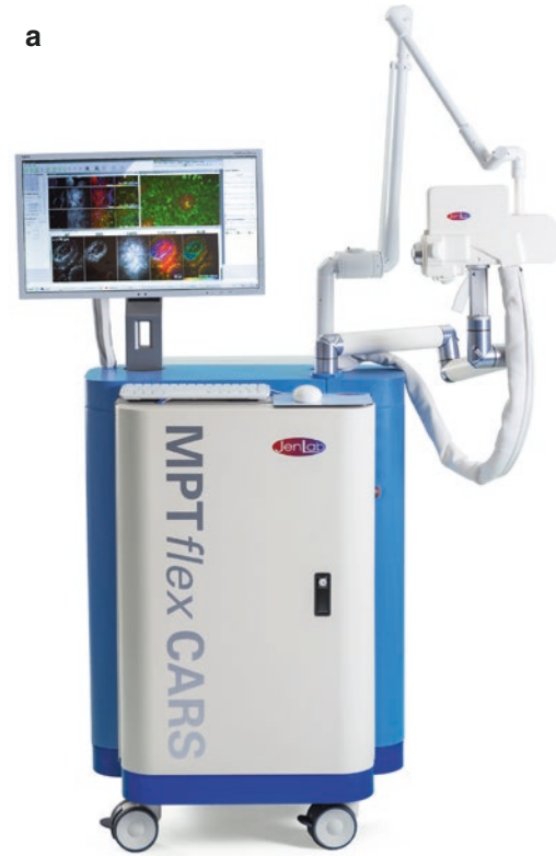
Fig. 4.13 A. MPTflex, a commercial clinical multiphoton microscope [235]. B. Multiphoton view of a pigmented lesion at a depth of 40 microns in skin: second harmonic generation (SHG—blue) from dermal collagen surrounded by pigmented keratinocytes visualized by two-photon fluorescence (green). Image taken at the Beckman Laser Institute, University of California, Irvine. Scale bar = 50 \mu\text{m}
