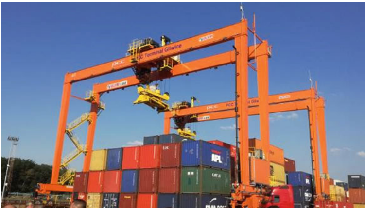
Fig. 15 Main bridge cranes for reloading of containers in Gliwice logistic centre
