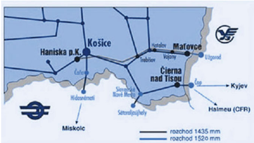
Fig. 21 Scheme of the East Slovakian transshipment area Čierna nad Tisou (ESTS). Source [29]
