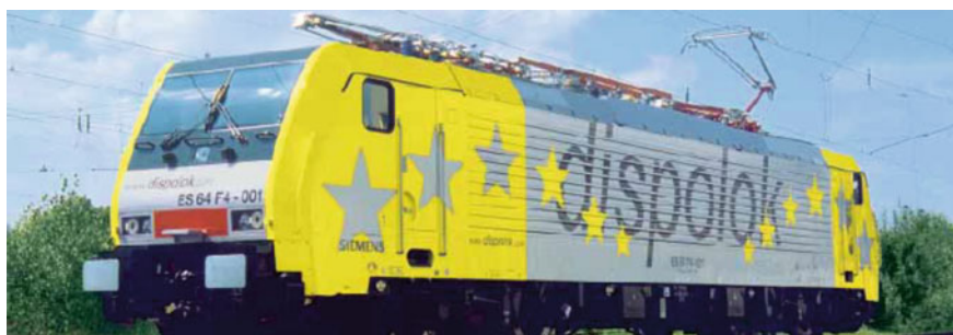
Fig. 24 Eurosprinter ES 64 F4. Four-system high performance locomotive. Source [42]
