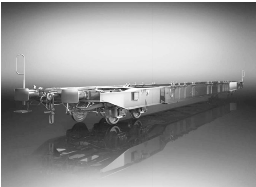
Fig. 25 Intermodal wagon Sggns 80'. Source [44]
