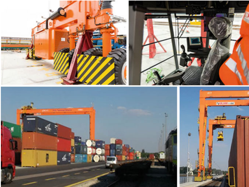
Fig. 17 Construction and basic elements of container gantry crane (RTG) in logistics centre in Gliwice
