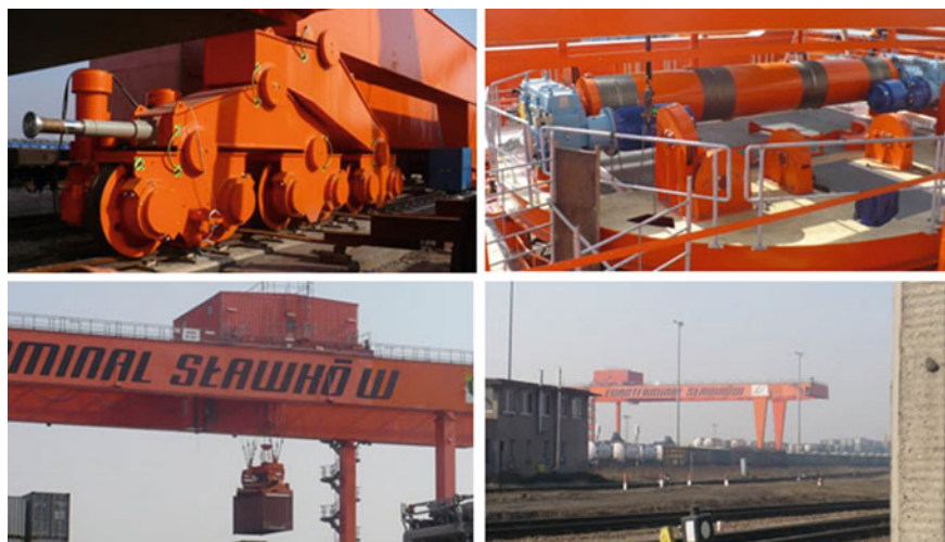
Fig. 16 Construction and basic elements of container gantry crane (RMG) in logistics centre in Sławków
