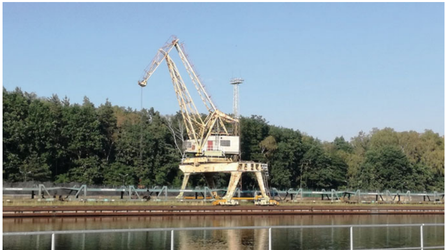
Fig. 10 Jib crane for bulk material handling in the Gliwice logistic centre
