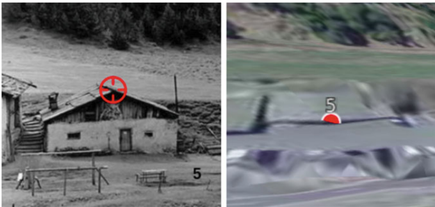
Fig. 5 Incorrect GCP provided on a building. The roof top is clicked in the image, while the same location is provided at ground level in the virtual globe
