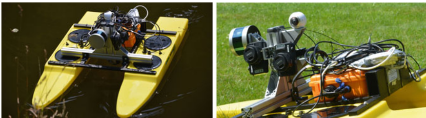
Fig. 1 Unmanned boat systems carrying laser scanners, cameras (RGB, infrared, 360°) and echo sounders (single beam)
