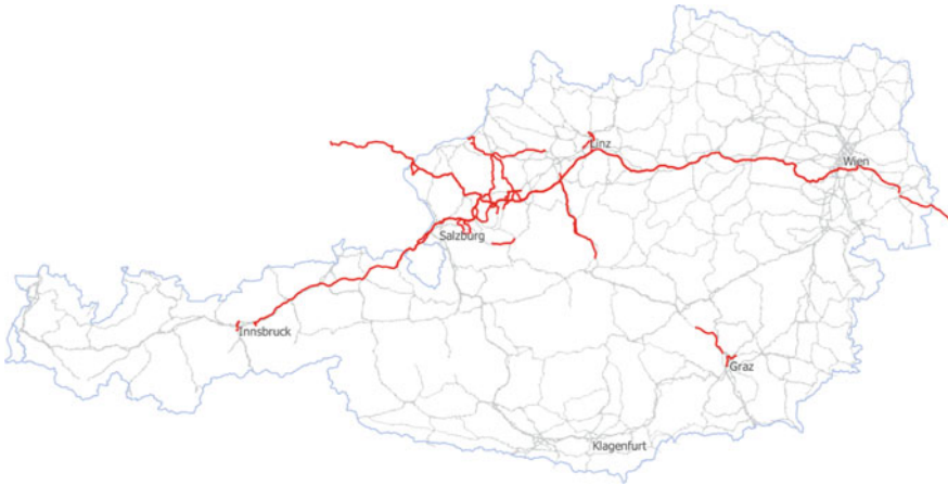
Fig. 7 32 GNSS trajectories (red lines) as sample data visualized on top of the Austrian OSM dataset (grey lines)
