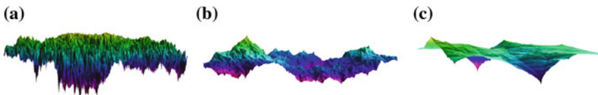
Fig. 2 Fractal terrains with different roughness values, r_a = 0.5 , r_b = 1.0 , r_c = 2.0
