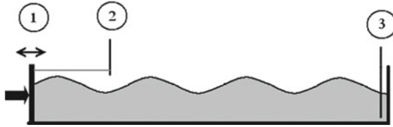
Fig. 1 The scheme of the experiments, (1) is the wavemaker, (2) is the transducer of horizontal displacement of wavemaker, (3) is the resistive probe of a free surface displacement
