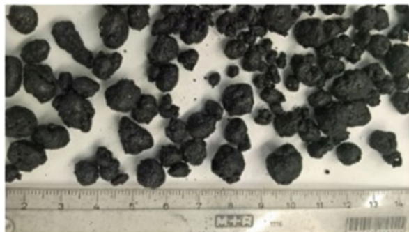
Fig. 73.1 The granulated Petrit-T using Eirich high-intensity mixer
