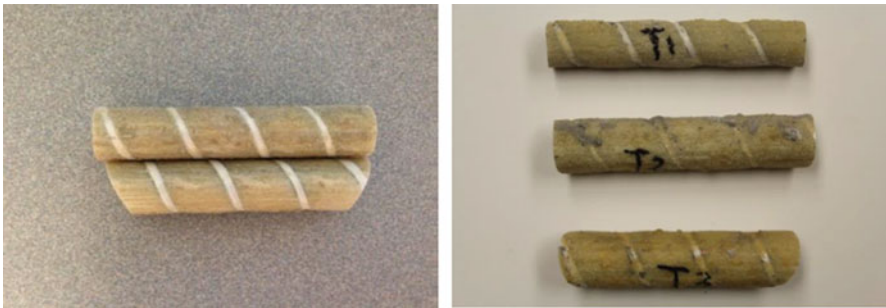
Fig. 75.1 The extracted GFRP samples from Southview Bridges (left) and Sierrita de la Cruz Bridge (right)
