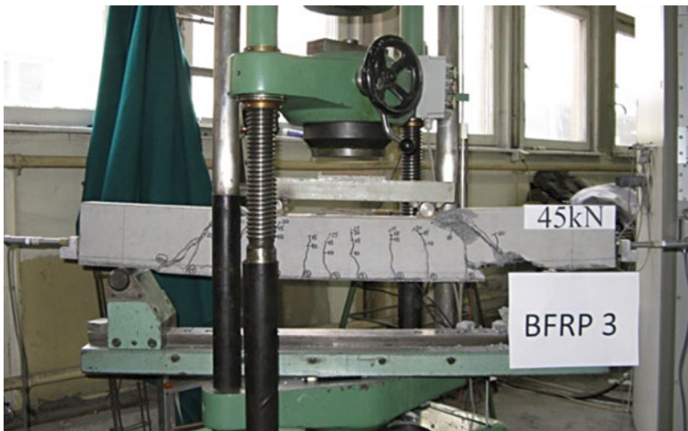
Fig. 85.2 Destruction of one of the samples reinforced with BFRP bars
