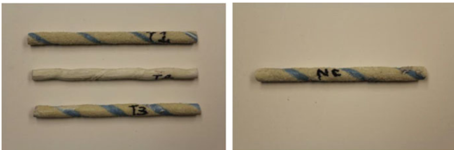
Fig. 75.2 The extracted GFRP samples from core1 (left) and core2 (right) of Walker Bridge
