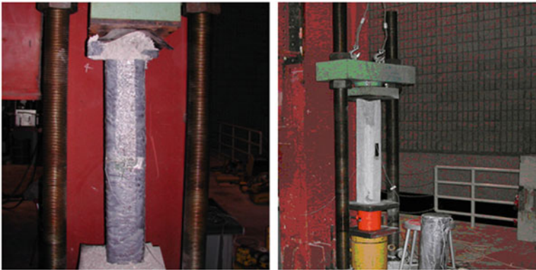
Fig. 93.2 Failure modes of confined and unconfined columns
