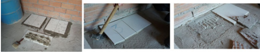
Fig. 58.2 Adhesion test of cementitious adhesive
