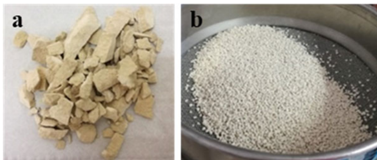
Fig. 23.1 Lecce Stone in flakes (a) and sieved Lecce Stone (b)
