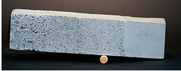
Fig. 1.12 Variable density concrete using 3-D printer [11]
