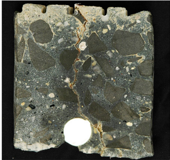
Fig. 2.4 Plastic shrinkage cracking (left); drying shrinkage cracking (right)
