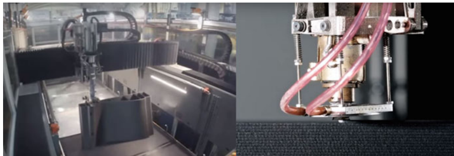
Fig. 12.4 3D printing of wind turbine blade molds using the Big Area Additive Manufacturing machine (US Department of Energy 2016)
