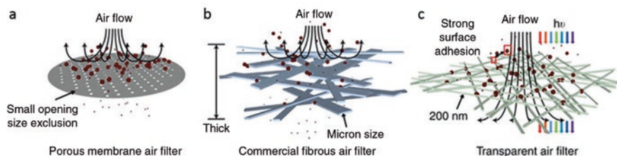
Fig. 9.4 Comparison of different air filters. (a) Schematic of a porous air filter capturing PM particles by size exclusion. (b) Schematic of a bulky fibrous air filter capturing PM particles by constraint and adhesion. (c) Schematic of transparent air filter that captures PM particles by strong surface adhesion whilst allowing high light and air penetration
